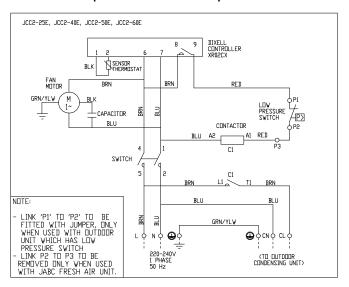
Note: Units manufactured from March 2015 are fitted with an extra terminal (P3) at the terminal block to provide a wiring connection point when used with JABC-1 Fresh Air Unit.
